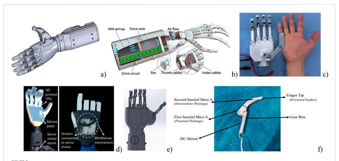
(a) Active prosthetic hand: Asto V.4 (Annanto et al., 2021); (b) Prosthetic hand with 19-DOF dexterity (Sankar et al., 2025); (c) Dexterous Prosthetic Hand (Zhang et al., 2022); (d) Single-Actuator Soft Robotic Prosthetic Hand (Mohammadi et al., 2025); (e) Low-Cost Biomechanical Hand Prosthesis (Krepsky et al., 2025); (f) Robotic finger with mechanical assemblies (Mughal and Mughal, 2023).
