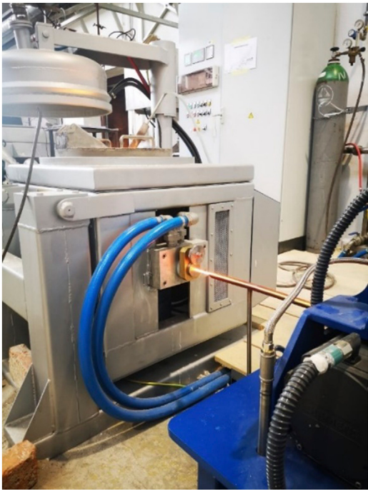
FIGURE 1 Induction furnace with horizontal continuous caster.
