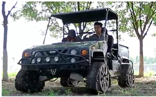
FIGURE 31 ATV equipped with variant wheel passing the grass terrain test.
