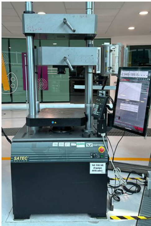
FIGURE 6 Universal test machine for traction tests.
