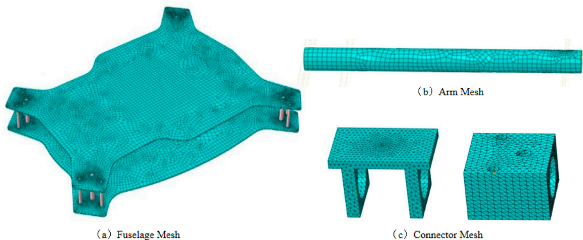
FIGURE 3 Mesh of UAV. (a) Fuselage mesh. (b) Arm mesh. (c) Connector mesh.
