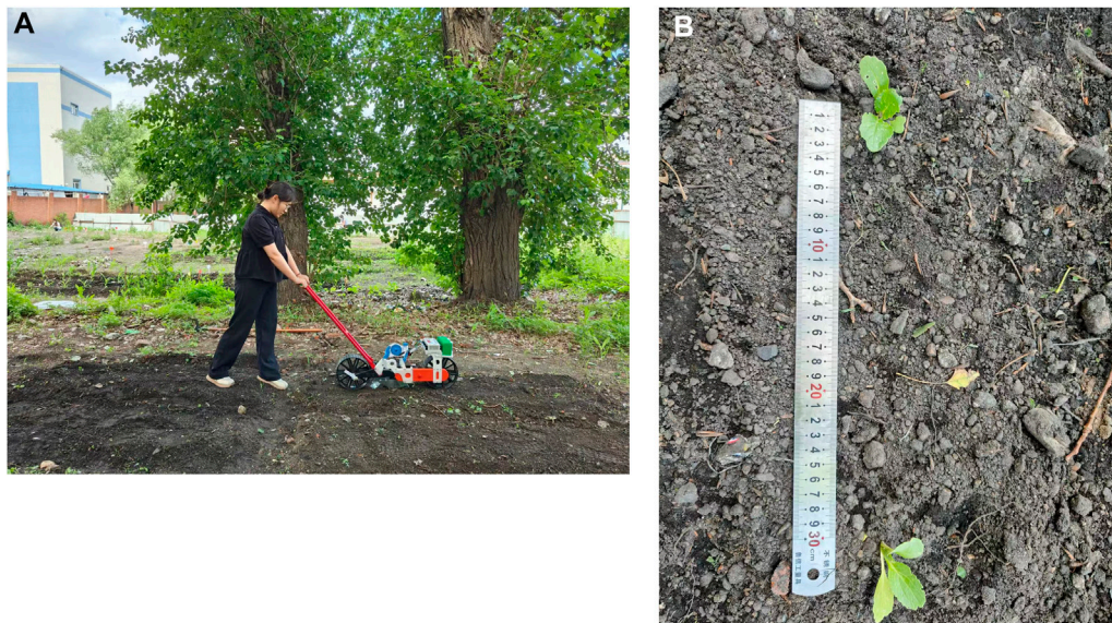
FIGURE 26 Field sowing test. (A) Field sowing trials. (B) Chinese cabbage seedling emergence effect.
