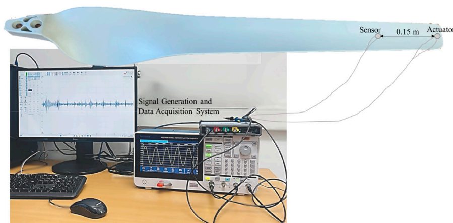
FIGURE 1 Experimental setup for guided wave-based inspection of WTB samples.
