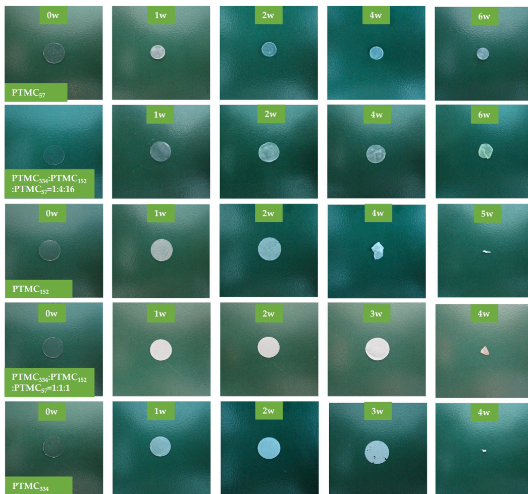
FIGURE 2 The macroscopic observation of the PTMC films PTMC films and ternary self-blending films at different times in 37 °C lipase.
