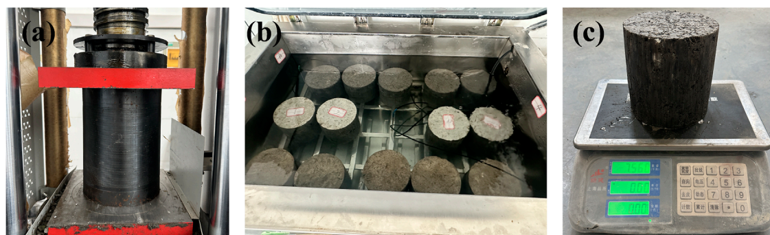
FIGURE 3 Freeze-thaw cycle test. (a) Specimen molding; (b) Freeze-thaw cycle test; (c) Weigh the quality.
