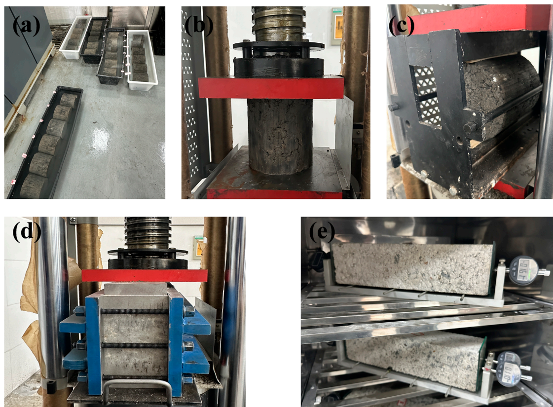
FIGURE 2 Performance Testing. (a) Soaking in water; (b) Unconfined compression test; (c) Splitting test; (d) Specimen molding; (e) Contraction test.
