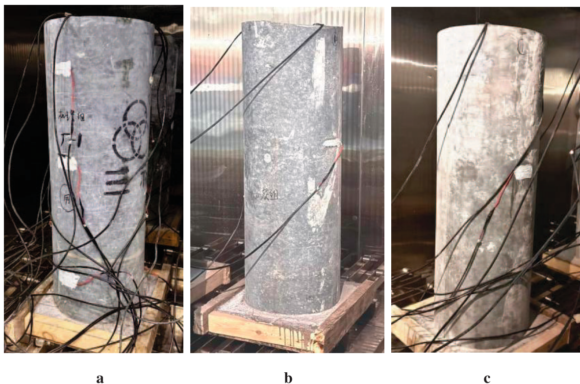
FIGURE 4 Pipe pile specimens. (a) Pipe Pile 1. (b) Pipe Pile 2. (c) Pipe Pile 3.
