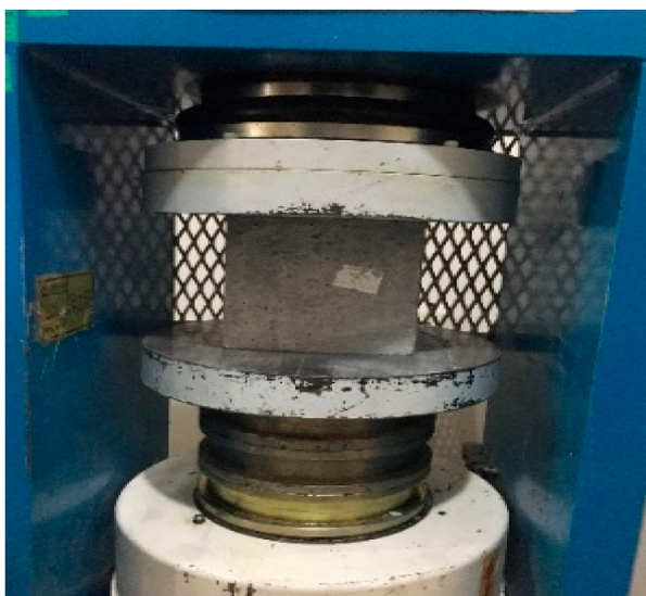
FIGURE 3 Concrete compressive strength test.
