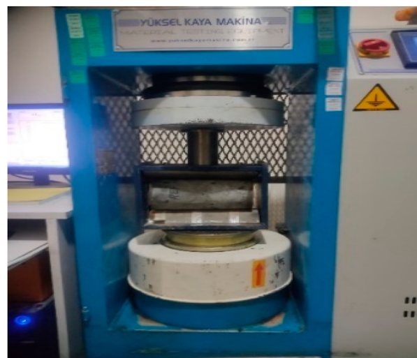
FIGURE 5 Concrete splitting tensile test.
