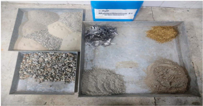
FIGURE 1 Materials used in hybrid steel fiber-reinforced concrete mixtures with fly ash.
