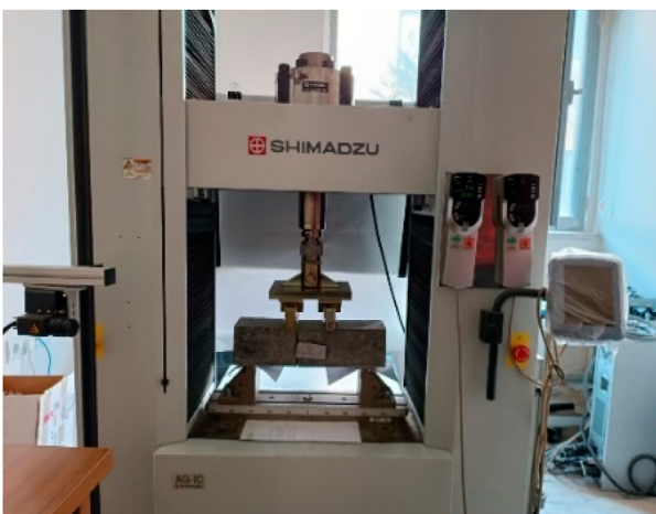
FIGURE 4 Beam flexural strength test.
