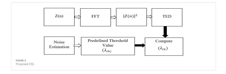
Here,  $\sigma_{Wn}$  and  $\sigma_{Ws}$  denote noise and signal variance, respectively. Finally, the  $E_{Th}$  is equated with the predefined threshold ( $\lambda_{TH}$ ) to indicate the availability and absence of the user. It is important to analyze the performance of the ESS by estimating parameters, such as Pd and Pfa.
