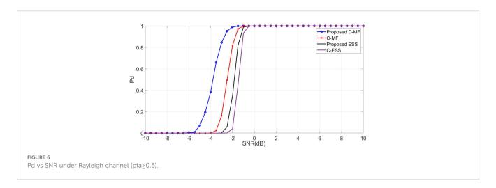
and high Pd, which leads to a better and more reliable use of the spectrum. The Pfa vs. Pd ratio for a Rician channel is shown in Figure 9. The maximum detection is obtained by the proposed DMF and ESS at Pfa of 0.1 and 0.17 as compared with 0.22 (C-MF) and 0.3 (C-ES). Hence, it was concluded that the proposed methods obtained efficient detection while minimizing the effect of false alarms.
