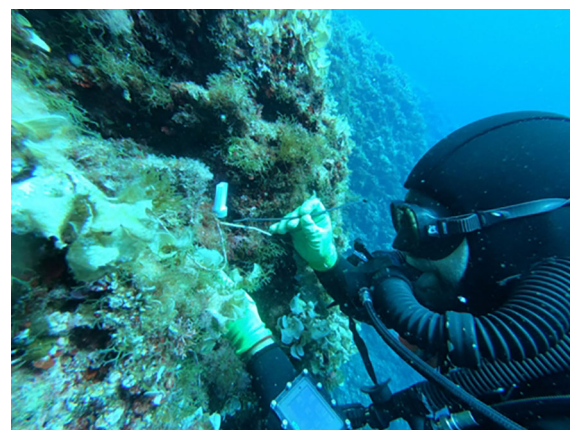
FIGURE 7 Underwater manual sensor mounting by diver.
