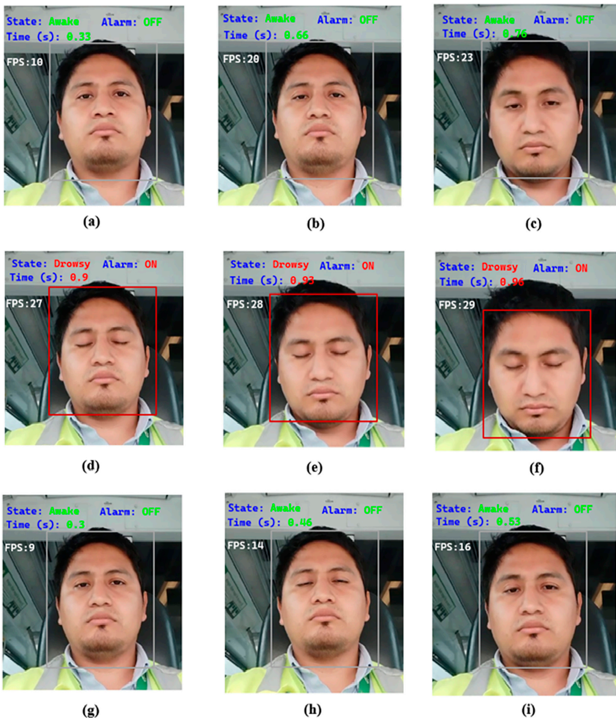
FIGURE 3 Drowsiness detection system inside a train. . (a) Frame 1. (b) Frame 1. (c) Frame 1. (d) Frame 1. (e) Frame 1. (f) Frame 1. (g) Frame 1. (h) Frame 1. (i) Frame 1.
