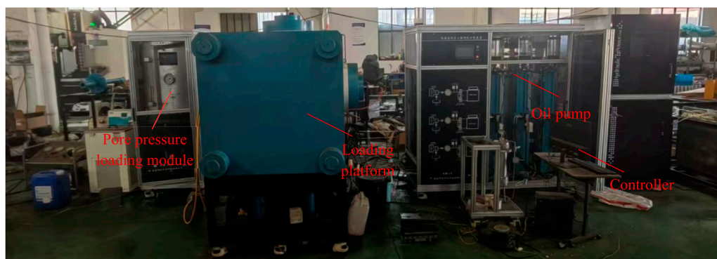
FIGURE 3 True three-axis hydraulic fracturing equipment.
