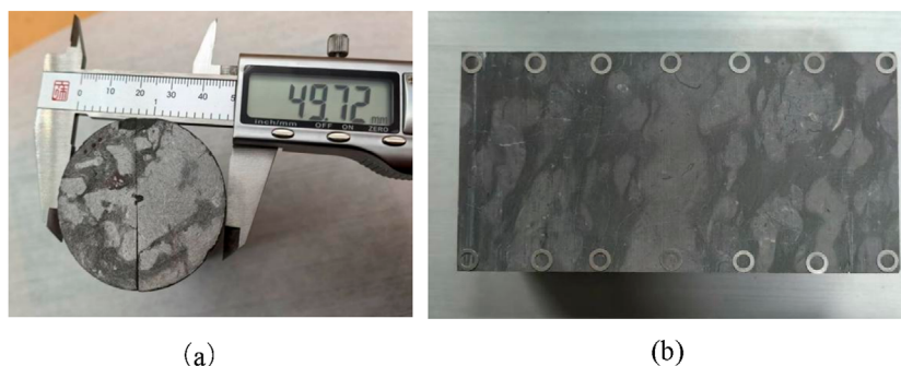
FIGURE 2 Morphology of dissolution specimens: (a) sample geometry; (b) configuration of initial fracture apertures.
