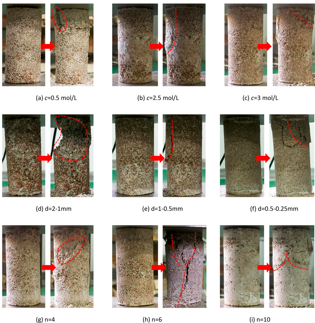
FIGURE 13 Failure modes of SICP-cemented samples from recycled construction aggregate. (a) c = 0.5 mol/L (b) c = 2.5 mol/L (c) c = 3 mol/L (d) d = 2-1 mm (e) d = 1-0.5 mm (f) d = 0.5-0.25 mm. (g) n = 4 (h) n = 6 (i) n = 10 .
