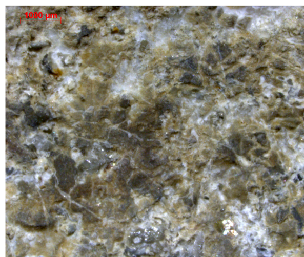
FIGURE 4 Surface of beached ACM waste fragment altered by subaerial organic corrosion, observed under stereomicroscope. See text for detailed discussion.
