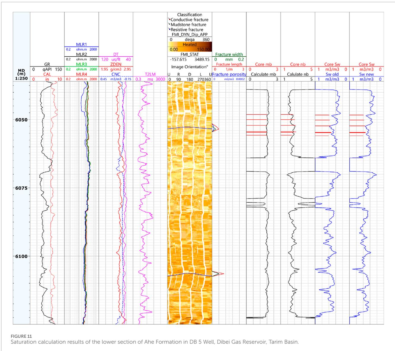
FIGURE 11 Saturation calculation results of the lower section of Ahe Formation in DB 5 Well, Dibe Gas Reservoir, Tarim Basin.
