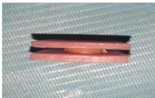
FIGURE 1 Tensile bond strength test assembly. Heat-cured polymethylmethacrylate (PMMA) plates are bonded to silicone denture soft liners (SDBSL).
