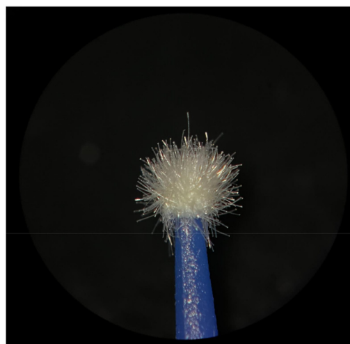
FIGURE 13 New KG Sorensen microapplicator.
