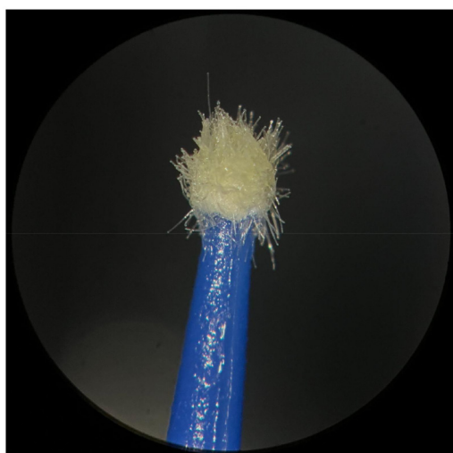
FIGURE 14 Used KG Sorensen microapplicator.
