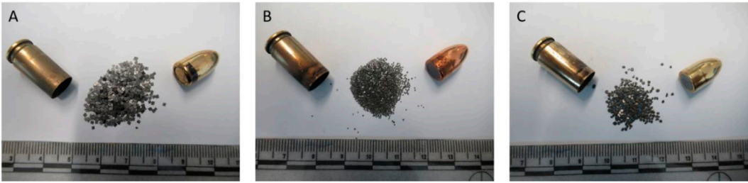
FIGURE 3 Cartridge case, bullet, gun powder and primer residue on the cartridge case of (A) Fiocchi NTA (B) ADCOM ammunition (C) NATO ammunition.
