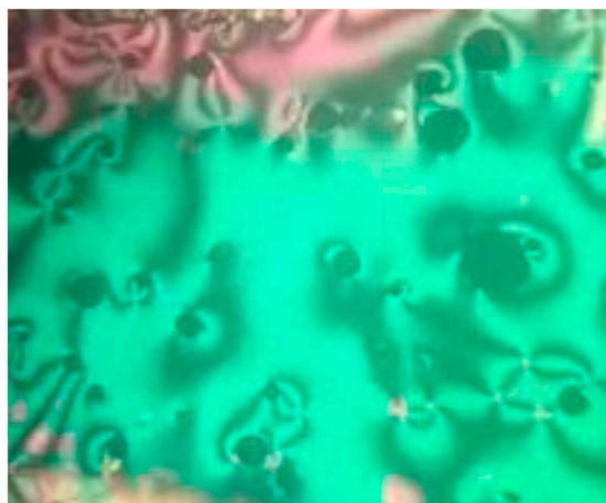
FIGURE 2 Textures observed under POM for compound M12 of (a) N phase at 120.0^\circ\text{C} upon heating and.
