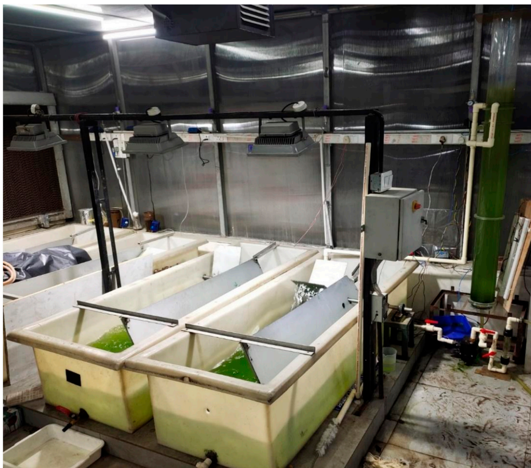
FIGURE 4 Modified raceway system hybridised with the carbonation column for real-time CO 2 assisted Poterioochromonas malhamensis cultivation. The unmodified raceway acted as control.
