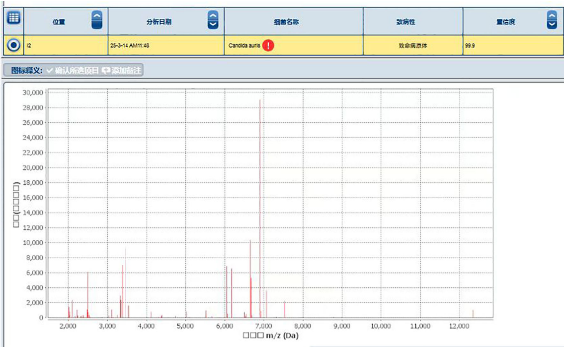
FIGURE 3 Identification of the Protein Fingerprint of C. auris strain CAS20503 Using MALDI-TOF MS. Peaks are visible across 2,000 to 12,000 m/z (Da) range, with significant peaks around 3,000 and 7,000 m/z, indicating protein masses.
