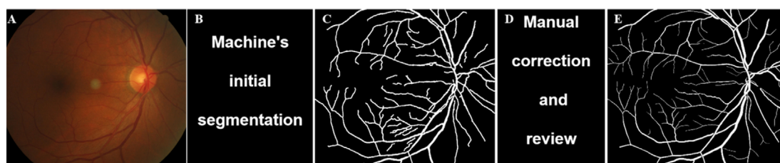
FIGURE 1 Vascular labeling process of fundus image. The specific process includes: (A) Original image; (B) Machine's initial segmentation; (C) Preselected vascular regions; (D) Manual correction and review; (E) Final labeled sample.
