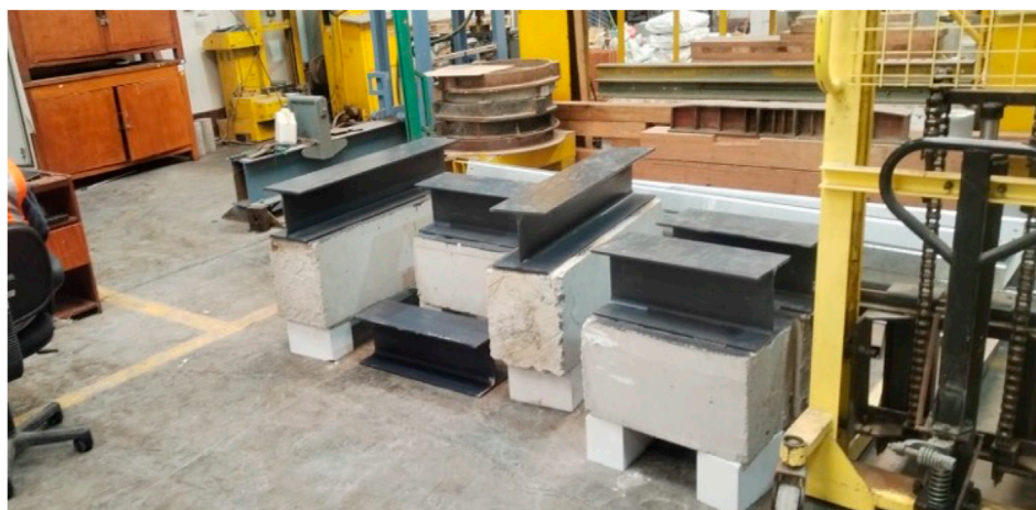
FIGURE 8 Representative samples adapted and prepared for laboratory testing, showing the integration of the H-profile with reinforced concrete elements.
