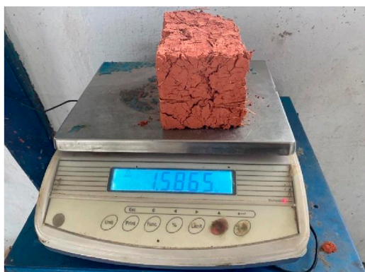
FIGURE 4 Weighing process of an adobe block.
