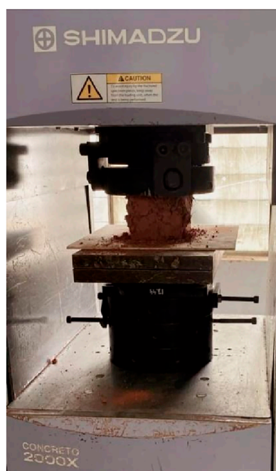
FIGURE 5 Compressive strength test of the adobe block.
