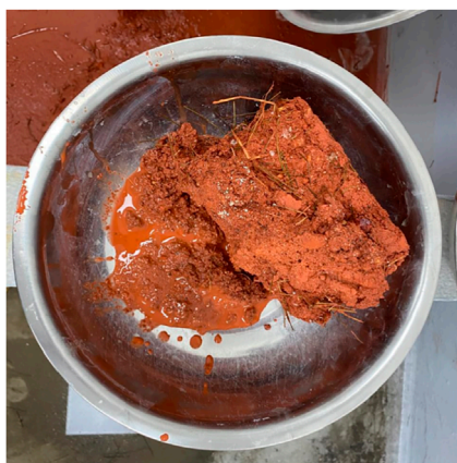
FIGURE 9 Post-fracture surface showing fiber anchorage and cohesive internal structure.
