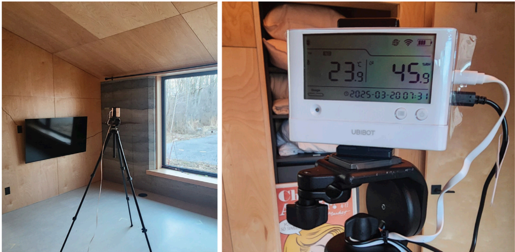
FIGURE 7 UbiBot device mounted on a tripod at the center of the Main room for temperature and RH monitoring.
