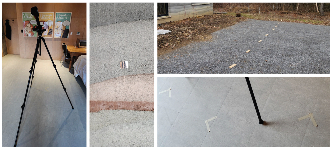
FIGURE 5 Monitoring setup for infrared thermography, illustrating the use of wall and floor markers to standardize image acquisition across all measurement intervals.
