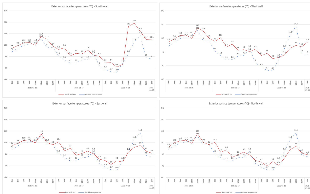
FIGURE 14 Exterior wall surface temperatures recorded via contact thermocouples embedded in heat flux sensors compared with ambient outdoor air temperature.
