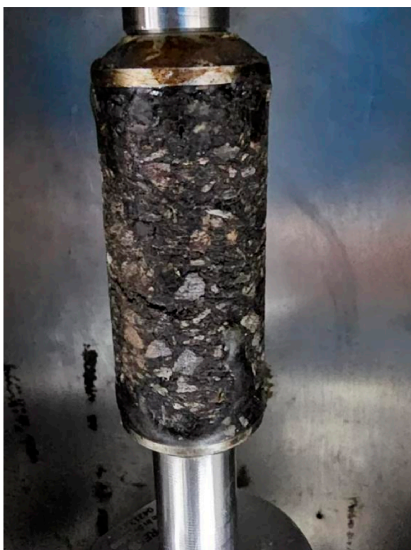
FIGURE 9 Fatigue test of AC-5 asphalt.
