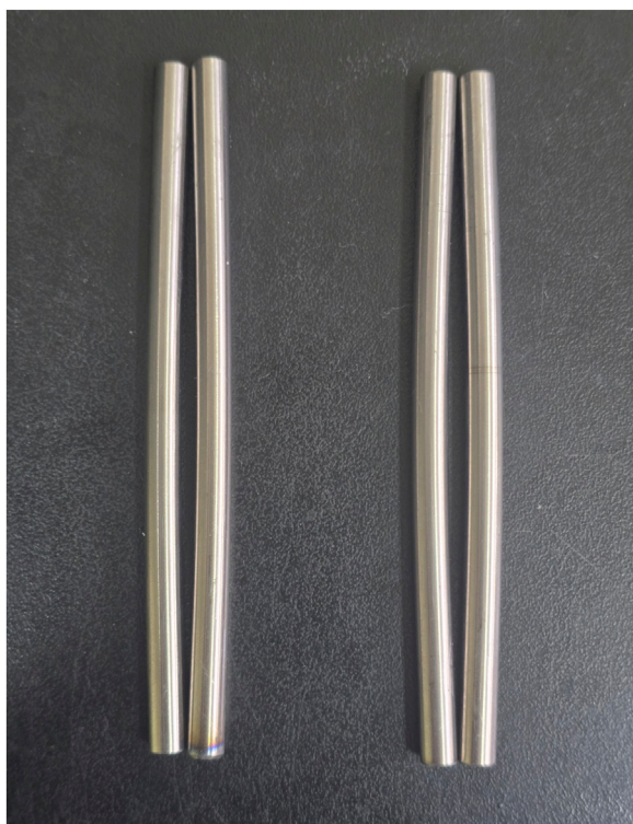
FIGURE 6 Permanently deformed spinal rods after 20 mm displacement in static compression and tension tests.
