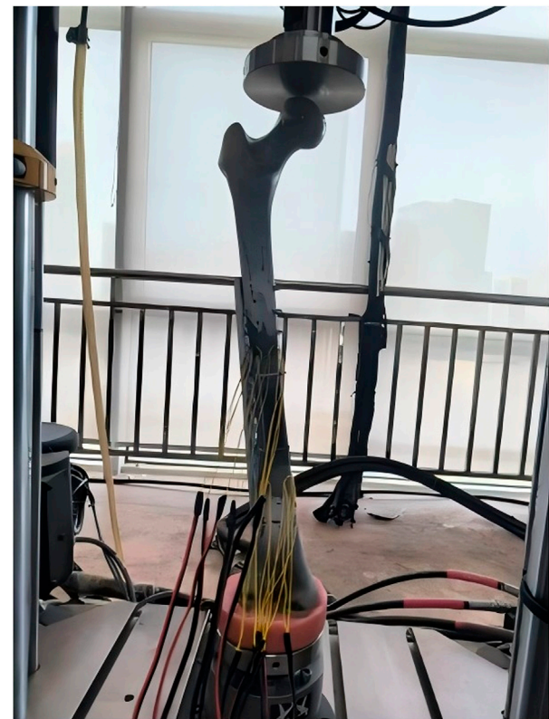
FIGURE 7 Detailed cyclic fatigue and failure test method: Sawbone model fixed into the test machine.
