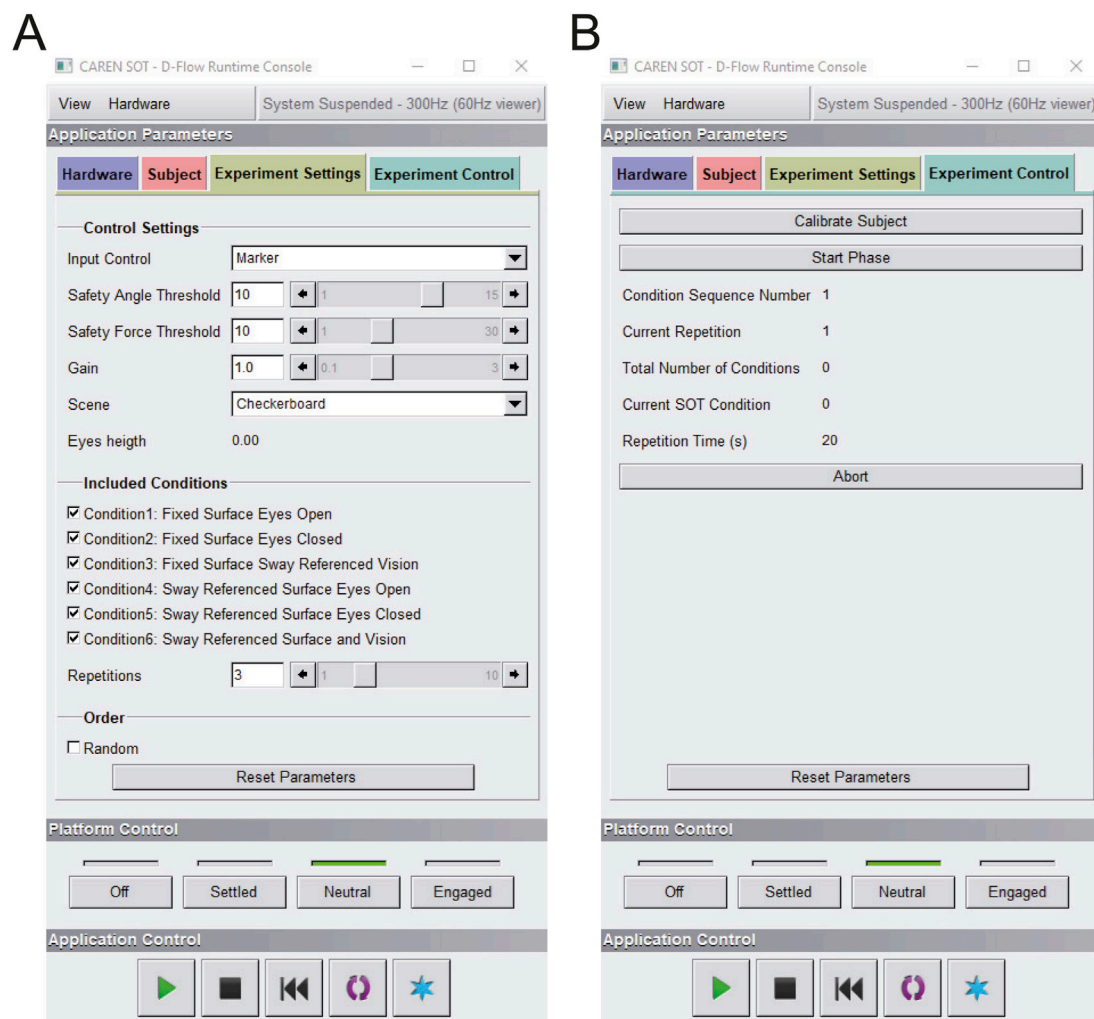
FIGURE 4 CAREN-SOT GUI (graphical user interface). (A) Experiment Settings tab: Interface for configuring experiment settings, including control parameters and conditions to be executed; (B) Experiment Control tab: Interface for executing the trials and monitoring the progress of the experiment.
