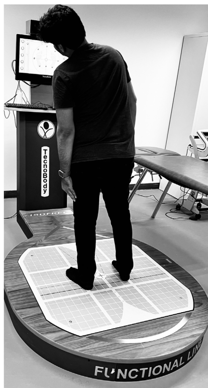
FIGURE 1 Limits of stability assessment using computerized stabilometric force platform.
