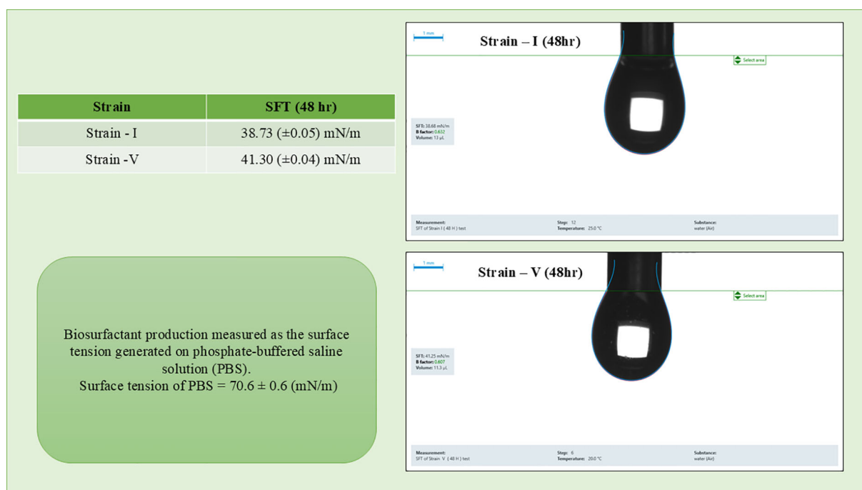
FIGURE 6 Surface tension reduction measurement comparing purified biosurfactants produced from Lactobacillus helveticus MTCC5463 and Lactobacillus rhamnosus MTCC5462.
