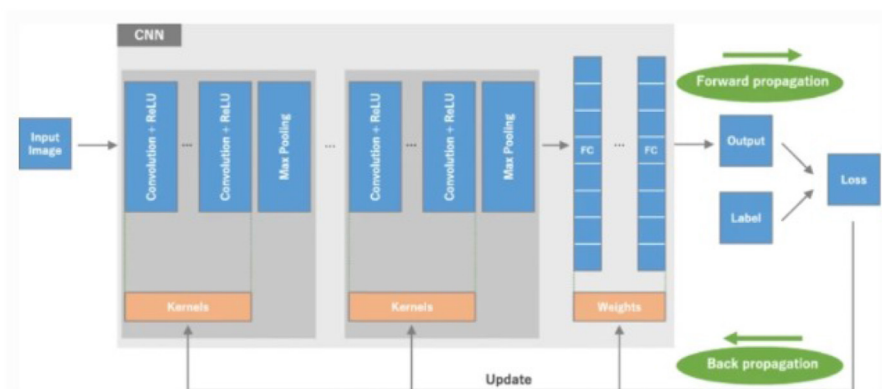
FIGURE 3 Architecture of CNN (Yamashita et al., 2018).
